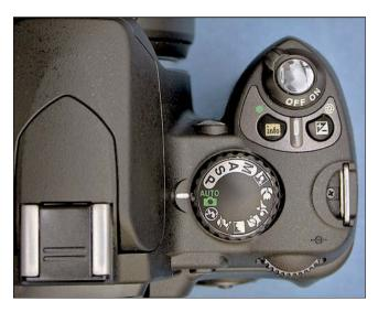
Figure 1-7: The tiny pictures on the Mode dial represent special automatic shooting modes.
