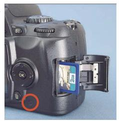
Figure 1-5: Insert the card with the label facing
