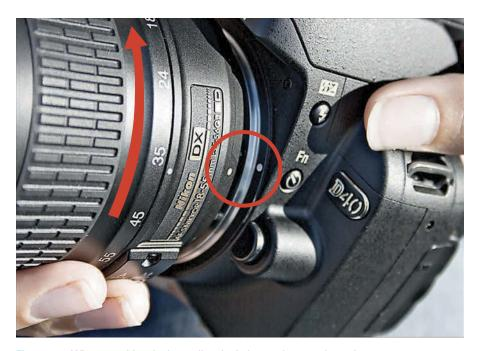
Figure 1-1: When attaching the lens, align the index markers as shown here.
