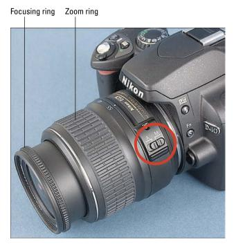
Figure 1-3: Set the focusing mode switch to M before turning the manual focus ring.
