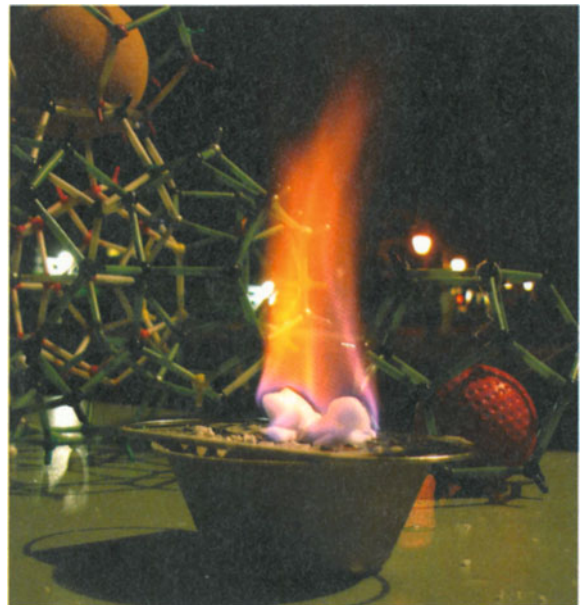
1.6 Combustion of a sample of synthetic methane hydrate. Laboratory investigations of methane hydrates will provide information on the utilization of these fossil fuels.
