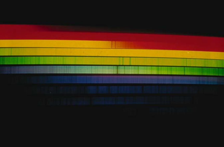
FIG. 1.6 Visible solar spectrum A spectrograph has spread out the visible portion of the Sun's radiation into its spectral components, displaying radiation intensity as a function of wavelength. When we pass from long wavelengths to shorter ones ( left to right, top to bottom ), the spectrum ranges from red through orange, yellow, green, blue and violet. Dark gaps in the spectrum, called Fraunhofer absorption lines, are due to absorption by atoms in the Sun. The wavelengths of these absorption lines can be used to identify the elements in the Sun, and the relative darkness of the lines helps establish the relative abundance of these elements. (Courtesy of National Solar Observatory, Sacramento Peak, NOAO.)
