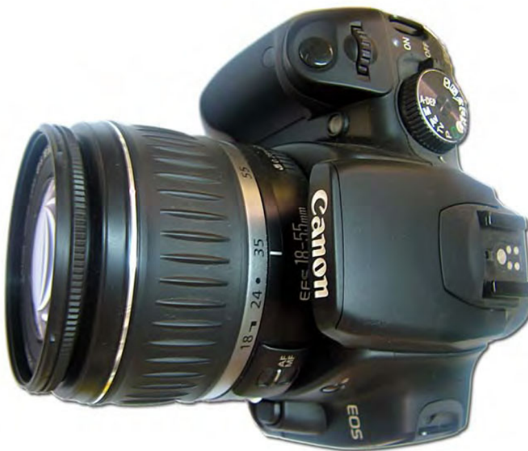
Figure 1-7. This image shows a digital single lens reflex camera with a lens mounted. This particular lens allows changing the focal length from 18 to 55 mm. The currently selected focal length is 35 mm.
