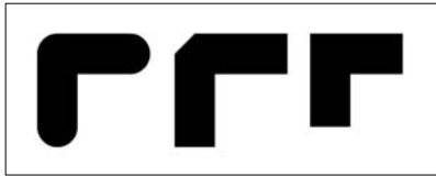
Figure 1-1. Three strokes with caps and joints set to ROUND on the left, SQUARE and BEVEL in the center, and NONE and MITER on the right
