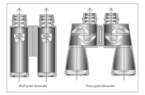
**Figure 2.1.** Optical light path through a roof prism binocular (left) and a Porro prism binocular (right). Although bulkier than the former, the latter is preferred for astronomical viewing because of its superior image quality.
