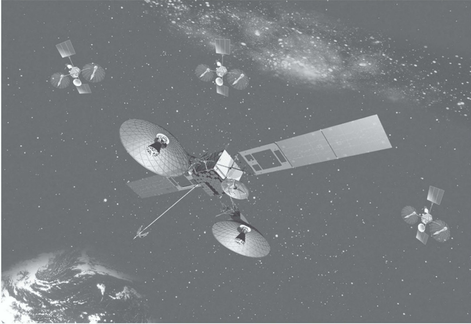
Figure 7. Artist's impression of four of NASA's TDRSS satellites in orbit. Each of its big dishes can communicate with a separate satellite in orbit far below. Credit: NASA.
