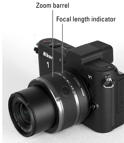
Figure 1-3: The focal length indicator tells you the current focal length of the zoom lens.
