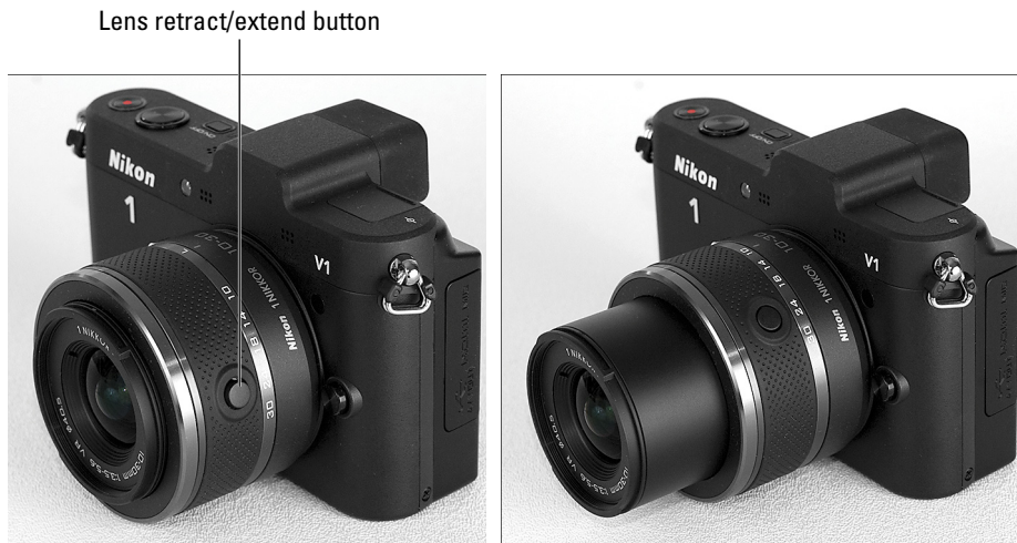
Figure 1-2: To extend and retract the lens, press the lens button while turning the zoom barrel.
