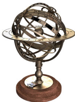
Fig. 1.4 A model of an armillary sphere. The spherical Earth is at the center. Depending on the latitude of the observer, the north-south axis of the Earth is inclined with respect to the horizon (the thick outside plate). Five rings perpendicular to the north-south axis are the Arctic Circle, Tropic of Cancer, the Equator, Tropic of Capricorn, and Antarctic Circle. The ecliptic (a thick band) is inclined 23.5^\circ with respect to the equator (Chap. 7, Vol. 1). Image created by the Technology-Enriched Learning Initiative of the University of Hong Kong
