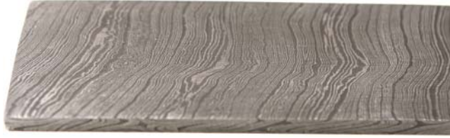
FIGURE 1.5 Damascene Steel The damascene sword techniques were believed to be first developed in India. Decorative etching and metal inlay methods were perfected in India in the first millennia BC. Source: L. William Zahner
