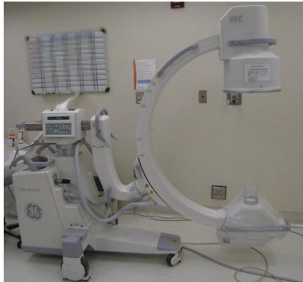
at one end and an X-ray receptor at the opposite end of the C-arm. The patient is placed on a radiolucent procedure table, between the X-ray tube and the receptor.
